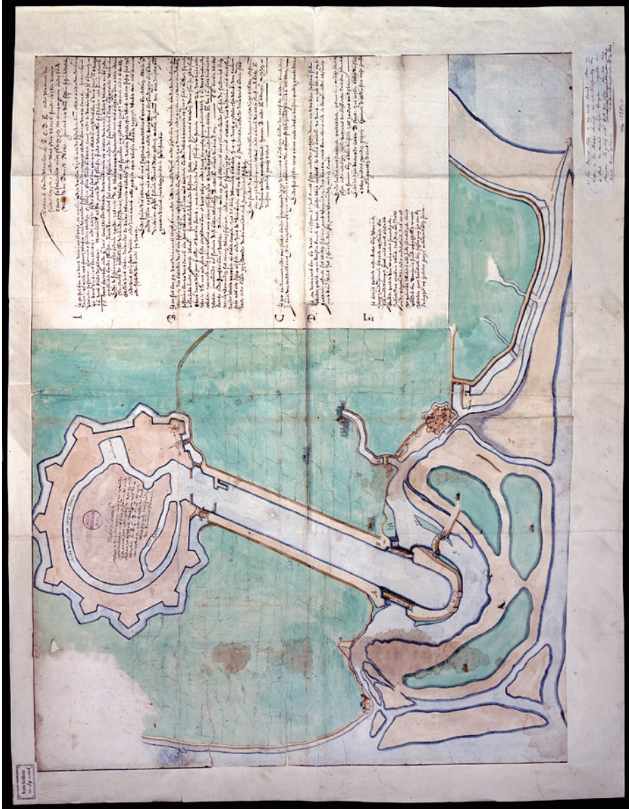
FIGURE 5.6 Daniel Note, design for floatable sluices to scour the harbour of Middelburg (1619–1620), ink drawing, 65 × 86 cm, mounted on paper 74 × 96 cm. Leiden University Library, Collection Bodel Nijenhuis 051-28-001.
