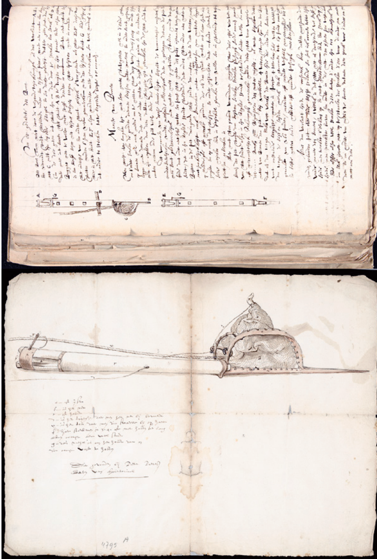
FIGURE 5.5A (Left) Pieter Pietersz Enten, drawing of drill as part of in 1602 granted patent for drilling deep in cities in Holland used in Amsterdam in 1605 [1602]. Ink, 393 × 58mm, The Hague, National Archives of the Netherlands, 4VTHR – 4795A.
