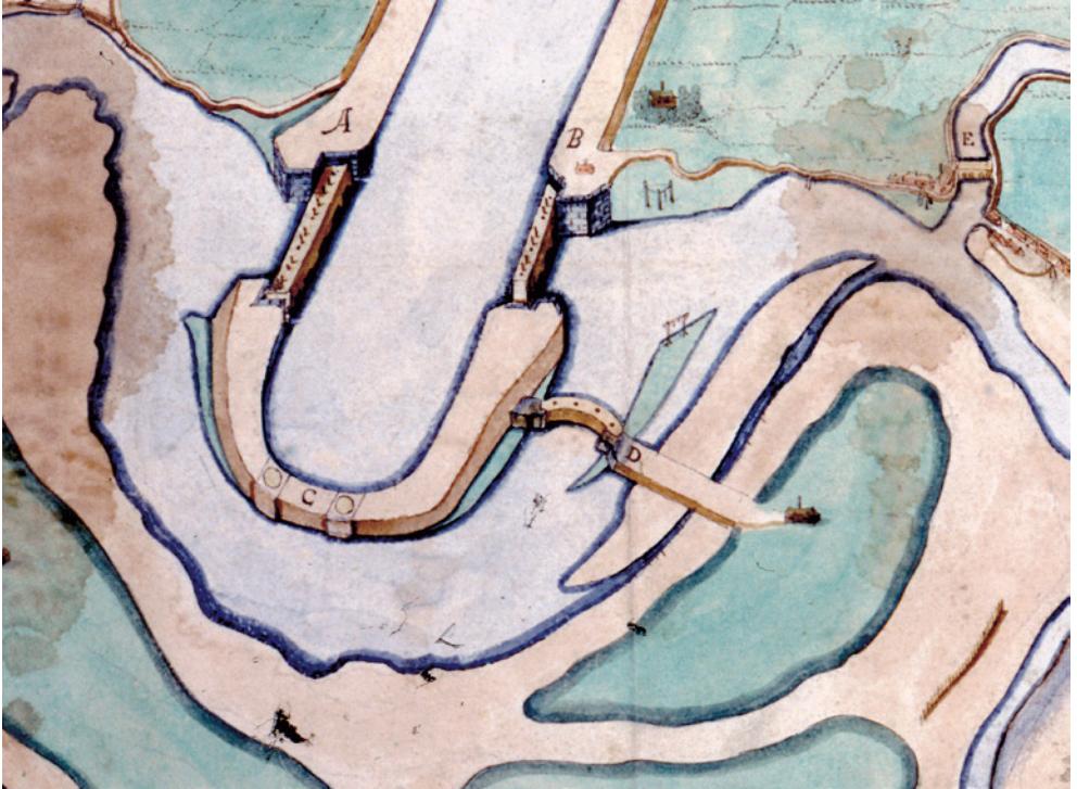
FIGURE 5.8 Daniel Note , design for floating sluices to scour the harbour of Middelburg (1619–1620). Manuscript map, 65 × 86 cm, mounted on paper 74 × 96 cm. Leiden University Library, Collection Bodel Nijenhuis 051-28-001. Detail, left below.
