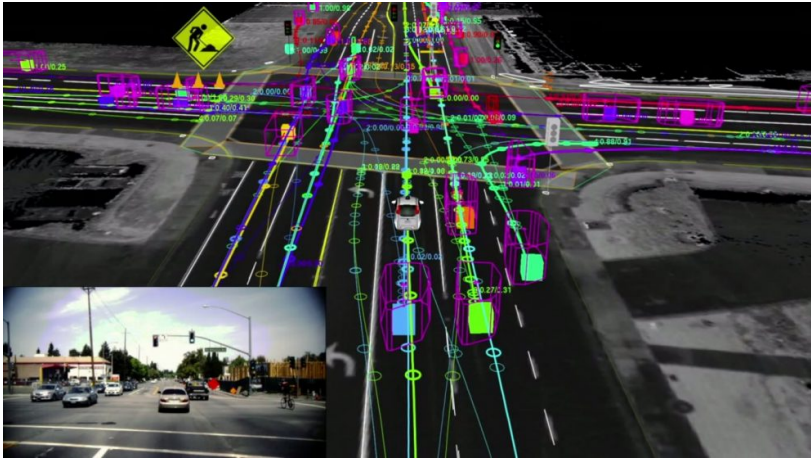
Figure 1.2: A typical intersection as seen by an autonomous vehicle. Future trajectories of the other vehicles are not known, but possible hypotheses can be made in a probabilistic fashion (graphic from [106], ©Waymo).
