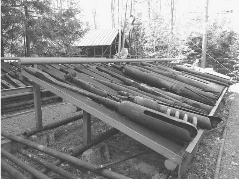
Figure 32: Drilling tools from a historic mine in Bóbrka. Source: Anna Kozicka-Kołaczkowska
