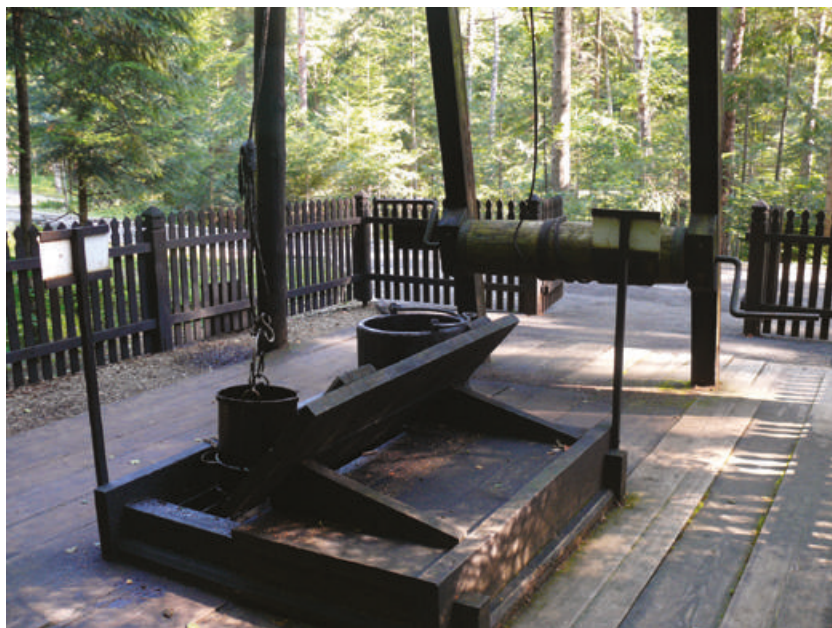
Figure 11: “Franek” manually dug well. Source: The Ignacy Łukasiewicz Oil and Gas Industry Museum in Bóbrka
