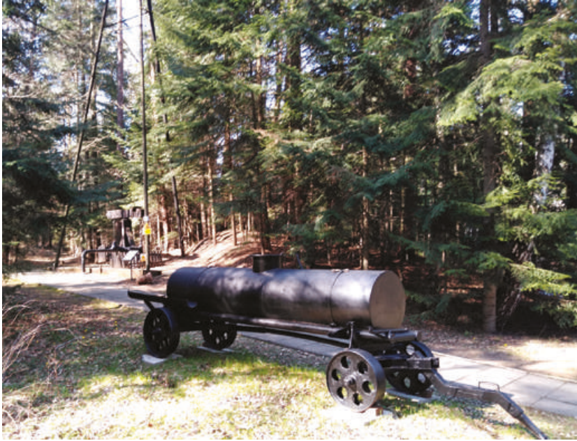
Figure 17: Vehicle for measuring the fluid extracted from a crude oil well from the 19th century. Source: Anna Kozicka-Kołaczowska.
