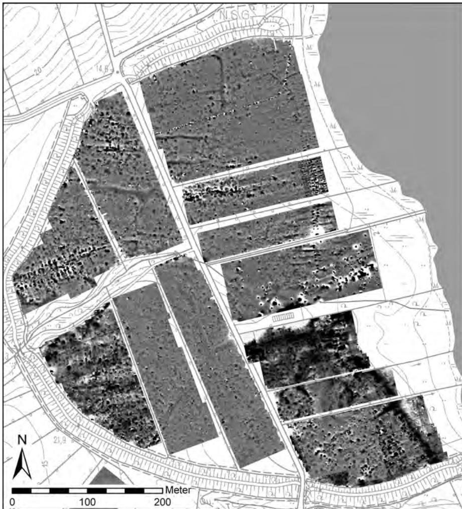
Fig. 3. Haithabu: Combined results of the magnetic survey in 2002 by the Marburg, Munich and Vienna teams. Dynamics ca. -10/+10 nT
