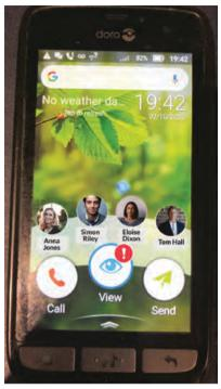
**Figure 7.6** Example of a Doro phone, showing its quick buttons for accessing important contacts. Photo by Daniel Miller.
