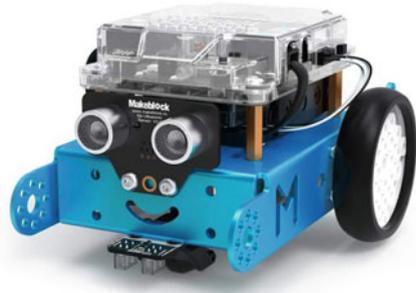
students can control the motor (wheels, belts, robotic arm) and can read and process the data measured by the robot's sensors, such as distance, brightness, direction, etc. [7].
