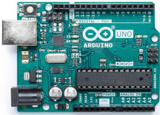
**Fig. 1** Front view of Arduino Uno board. Analog pins are numbered from A0 to A5 (bottom right), whereas digital pins go from 0 to 13 (top row). The symbol “~” denotes pins that can deliver an analog voltage by means of the pulse width modulation (PWM) technique
