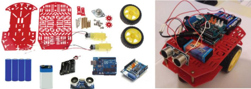
**Fig. 3** Basic components of a rover (left) and the final result after assembly (right)
