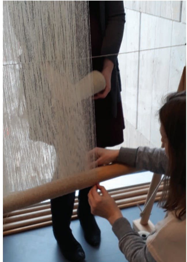
Fig. 10.8. Warping a two-beam loom with a tubular warp. Weaver Ulrikka Mokdad arranges the warp threads around the lower beam. Photo: Author.
