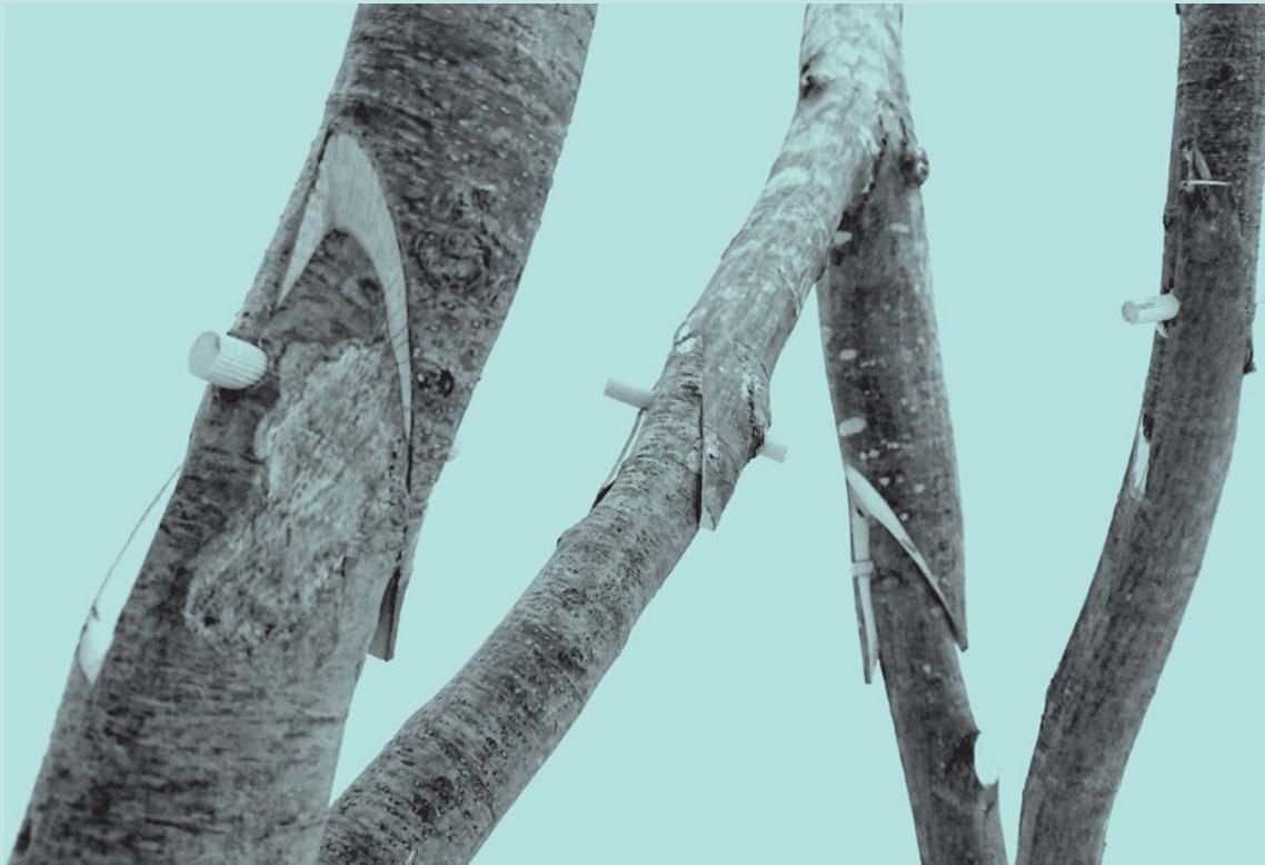
▲ Detail of the 'interlocking scarf joints' of the first robotic production of one tetrahedron module from branches.
