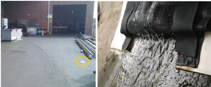
Figure 19.2 (a) Example of a polluting external yard area with the surface water drain circled; and (b) Kingston's extensive stormwater quality monitoring survey trialled the use of GAC absorptive media (Photos: T. Barrett).
