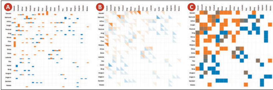
Fig. 13: Three different visual encodings for the comparison mode of the adjacency matrix: (A) juxtaposed color-coded bar charts, (B) split crosswise cells, and (C) color transition.
