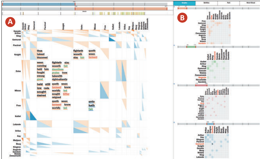
Fig. 14: (A) Our focus+context approach in the comparison mode with two different selected parts of the romance Parzival . (B) The graph desktop containing four user-selected graphs.
