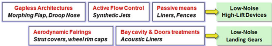
Fig. 10 Scope of investigated airframe noise solutions in CLEAN SKY
