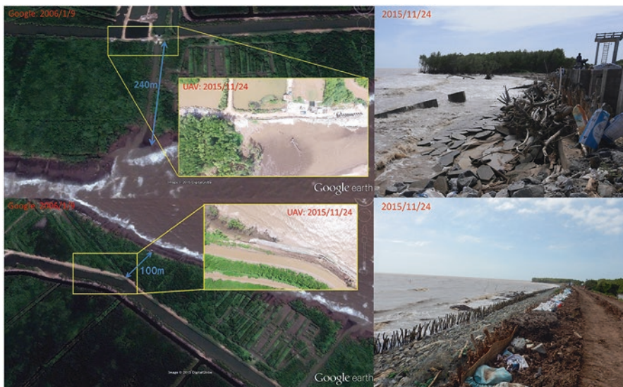
Fig. C3.2 Change in coastlines at the commune of Vinh Chau, Soc Trang (Tamura et al. 2018)
