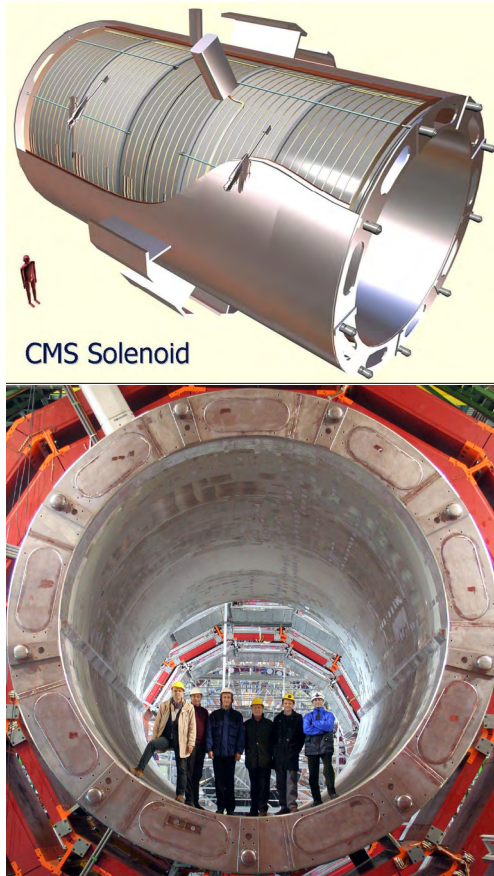
Fig. 3.10. (Upper) The CMS superconducting solenoid provides a central magnetic field of 4 T; the nominal current is 20,000 A, the weight of the cold mass is 220 tons, its length is 12.5 m and its diameter is 6 m; with stored energy 2.7 GJ it is the highest stored energy solenoid. (Lower) Members of the CMS Magnet and Integration Group and representatives from Saclay stand inside the cryostat of the giant superconducting solenoid during cooling to the interior operating temperature of 4.5 K (February 2006, Image reproduced with permission from CERN).
