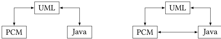
Figure 1.7.: Different transformation network topologies between PCM, UML and Java.
