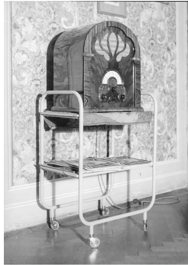
Fig. 116: Radio set with six tubes and loudspeaker by the brand Berliner from 1933. Source: Austrian National Library, 223.153-B.
