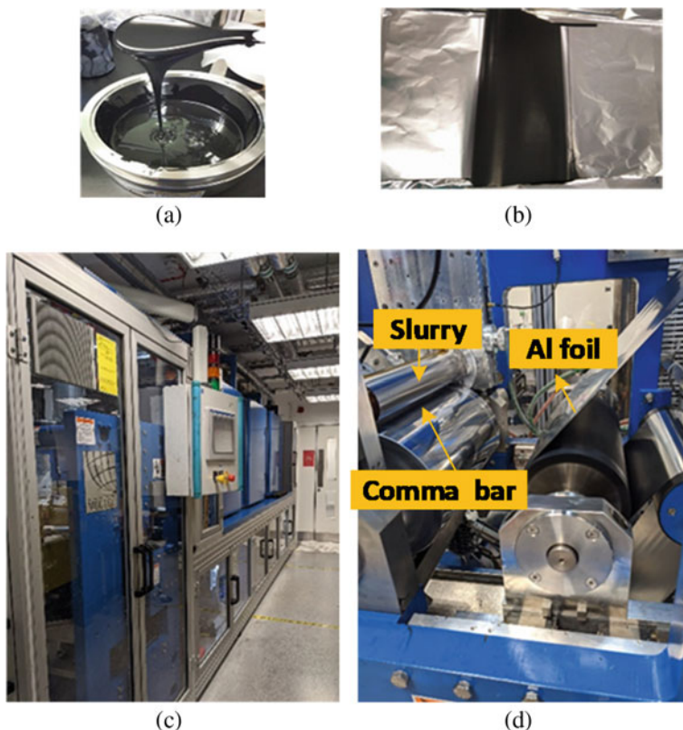
Fig. 2.3 Battery electrode manufacturing line: a slurry mixture, b coated foil, c electrode manufacturing machine, d coating machine
