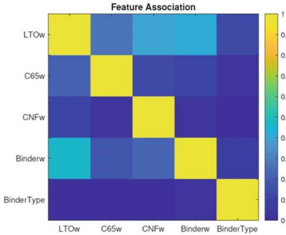
Fig. 3.29 Feature association for LTO capacity classification case, reprinted from [44], with permission from IEEE
