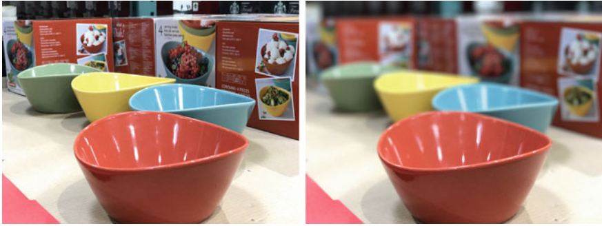
Fig. 3.1 (Left) For a close-in scene captured by a smartphone with a small aperture, all parts of the image will appear in focus. (Right) In order to mimic the aesthetically pleasing properties of a DSLR with a wide aperture, computational cameras now include a ‘portrait mode’ that blurs the background so the foreground stands out better
