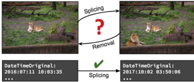
Fig. 15.17 Usage of metadata information to refine the direction of pairwise image provenance relationships. For the presented images, the executed manipulation operation could be either the splicing or the removal of the male lion. According to the image generation date metadata, the operation is revealed to be a splice since the image on the left is older. Adapted from Aparna Bharati et al. (2019)
