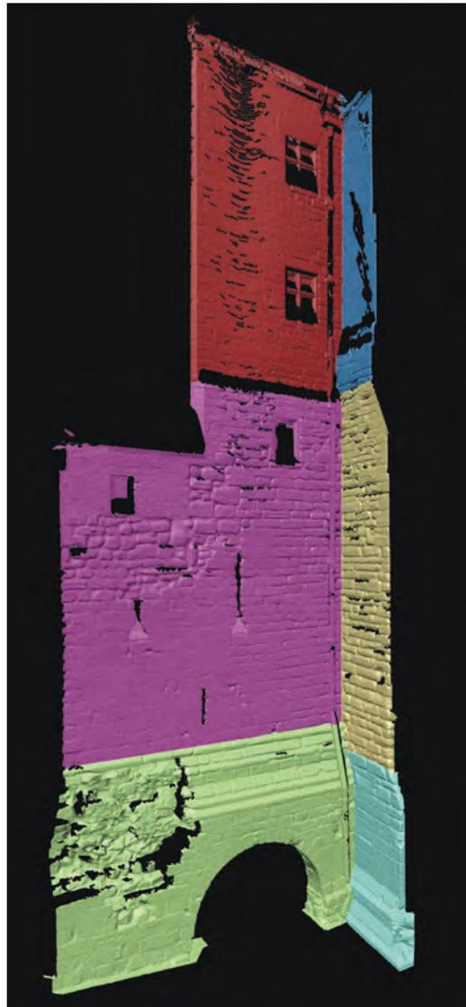
Fig 1.5 Laser scan survey of the Black Gate, 2009 (collaboration with the University of Northumbria, School of the Built Environment).
