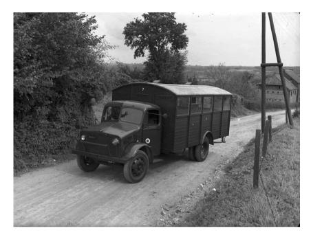
Figure 5: A Bedford truck repurposed into an emergency bus for transporting miners. N.p., 1945 (Source: Regionaal Historisch Centrum Limburg, Fotocollectie DSM, PR27, Creative Commons: BY-NC-SA)
