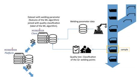
Fig. 9 Data collection and processing in federated learning environment
