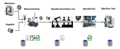
Fig. 8 GF milling machine spindles assembly process
