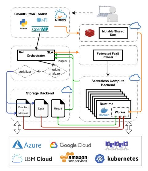
Fig. 2 CloudButton architecture
