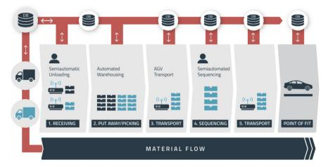
Fig. 6 System flow of data-driven intra-logistic 4.0 process
