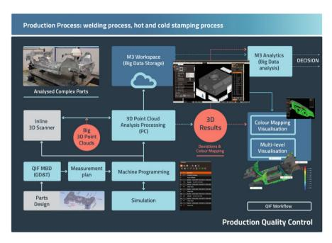
Fig. 18 QIF-ready semantic massive metrology big data analytics pipeline based on M3 platform
