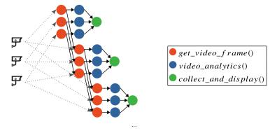
Fig. 4 DAG representation of the COMPSs example in Fig. 3
