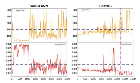
Fig. 2 Tutor4RL Performance compared to Vanilla DQN [20]. DO performance to manage 2 SLOs: costPerHour <0.03 and responseTime <200. Vanilla DQN is shown on the left, while Tutor4RL, with 2 guides and 1 constrain, is shown on the right. The horizontal blue dashed lines show the SLO threshold for the metrics and the pink dotted line show the moment in which guides are not used anymore
