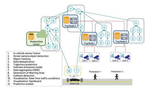
Fig. 8 Example of big data analytics distribution on the MASA and vehicles infrastructure
