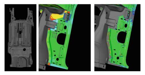
$\begin{tabular}{ll} Fig.~19 & Large-scale CAD file (left), annotated polygonal colormap mesh (middle), texturized colormap mesh (right) \\ \end{tabular}$
