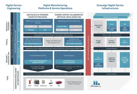
Fig. 11 +GF+ service development architecture
