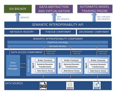
Fig. 2 Data Access and semantic interoperability Layer components of DataPorts Platform
