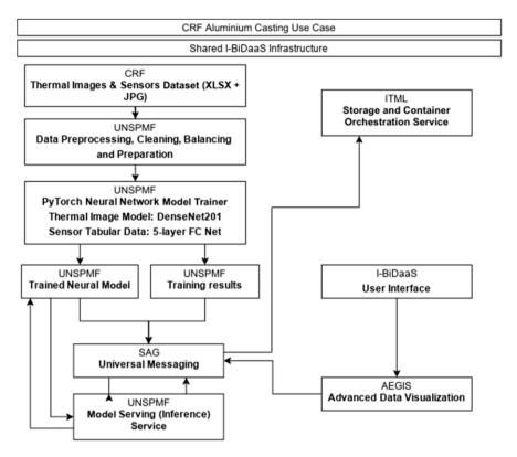
Fig. 2 Architecture of the 'production process of aluminium die-casting' use case
