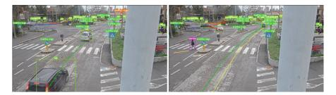
Fig. 4 Object tracking output from street camera detections
