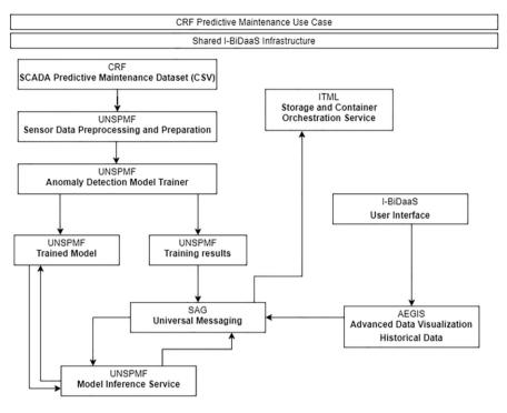
Fig. 6 Architecture of the 'maintenance and monitoring of production assets' use case
