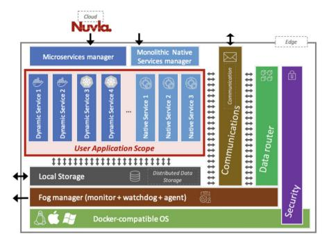
Fig. 6 Hybrid Fog Architecture
