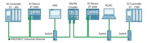
Fig. 9 Coupling of the PROFINET subnets with the PN/PN Coupler
