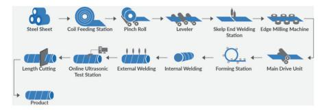
Fig. 3 Spiral welded steel pipe process
