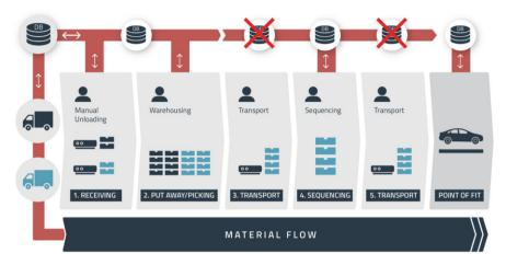
Fig. 5 Intra-logistic silo-based system flow of current process
