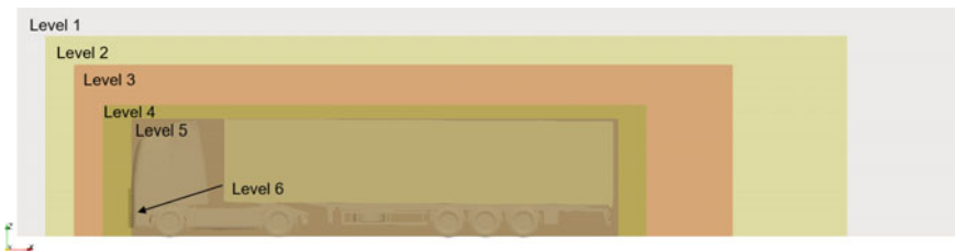
Fig. 5.4 Arrangement of the refinement boxes for meshing
