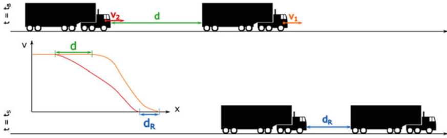
Fig. 9.2 Safe braking within a platoon. Starting from an initial distance d and initial speeds v_1 and v_2 at time t_B , each truck decelerates according to its deceleration capacity. A positive residual distance d_R at time t_S indicates that a collision can be avoided
