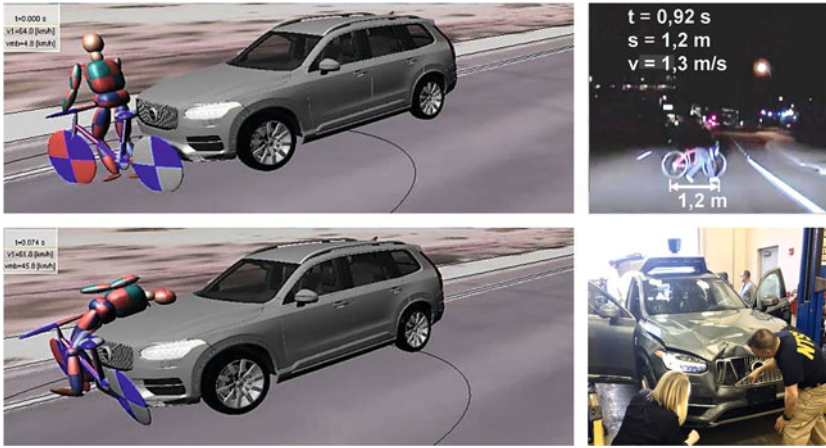
Fig. 4.5 Uber accident impact simulation with PC Crash and multi-body model. (Source: Winkle, PC-Crash accident reconstruction software, Google Maps, Tempe Police Station)
