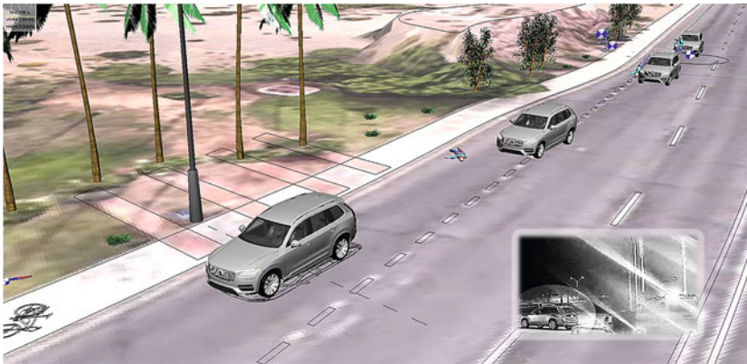
Fig. 4.4 Uber self-driving car accident reconstruction and original final position. (Source: Winkle, PC-Crash accident reconstruction software, Google Maps, Tempe Police Station)
