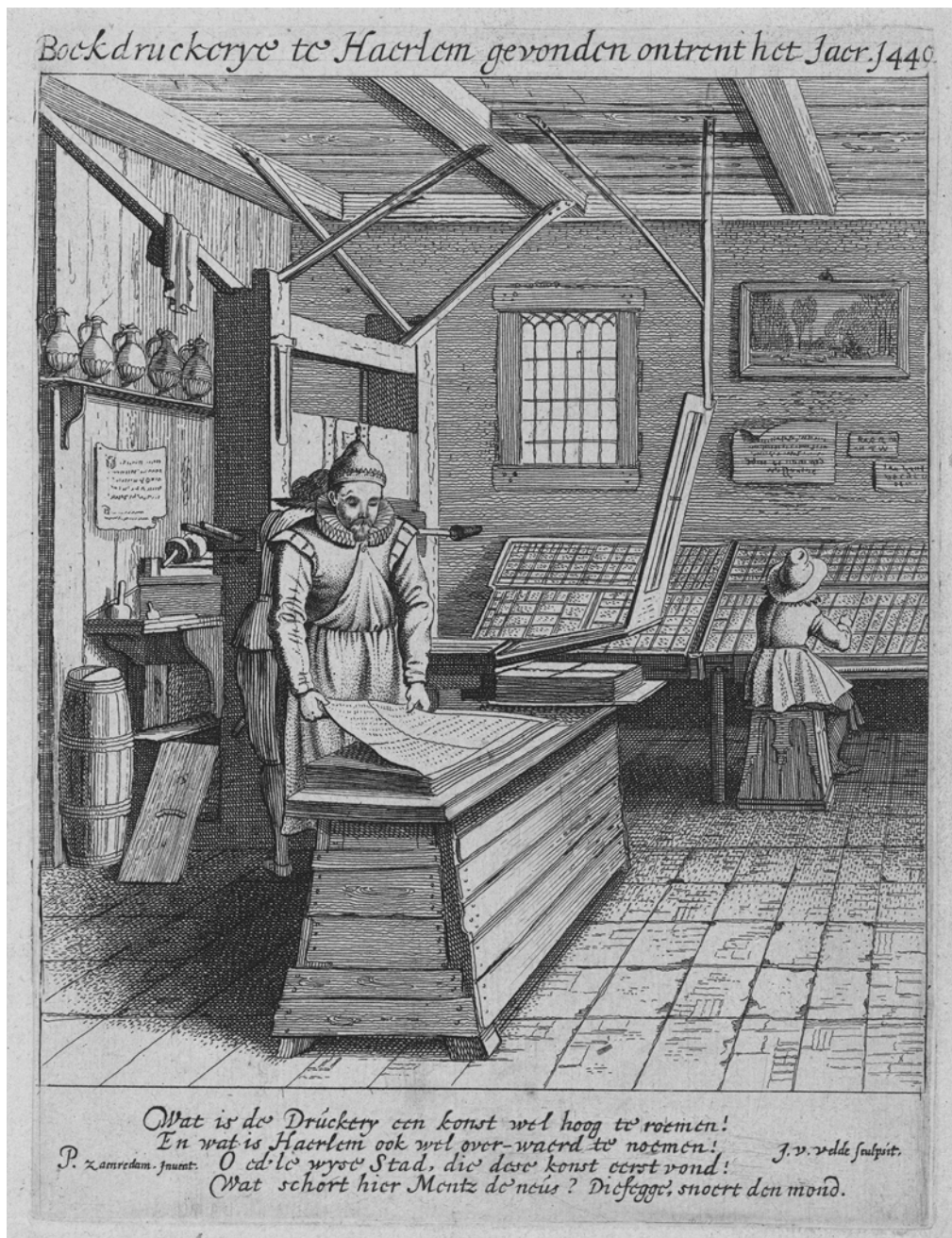
ILLUSTRATION 1.1 Interior (copper engraving, 1628) of a printing house in Haarlem in full operation. At the right a typesetter is composing pages. The printer at the left is busy printing imposed sheets at the handpress which are accordingly gathered and inspected by his assistant. At the outer left ink balls are lying on a cupboard. Presumably, the jugs standing on the shelf are containing ink.
