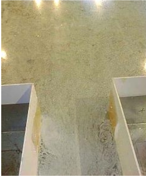
Figure 3.32: Picture of the pattern of flow field during the flood phase. Notice the presence of vortices in the left side of the channel inlet
