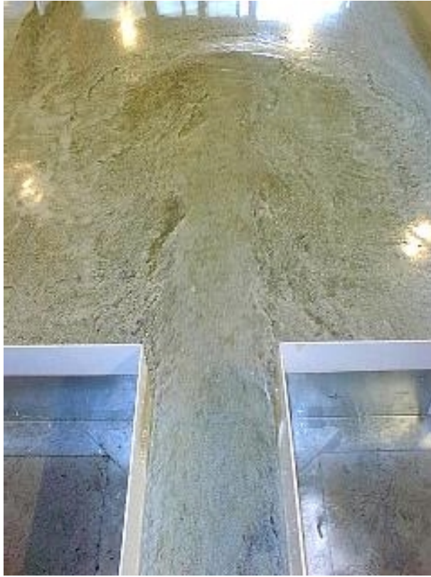
Figure 3.31: Picture of the pattern of flow field during the ebb phase
