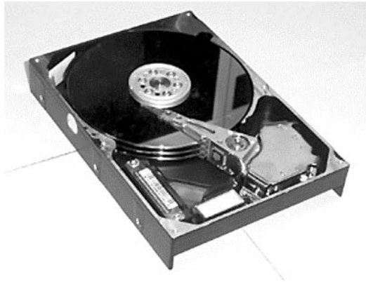
Figure 4. Image of hard drive with cover removed to reveal magnetic disk, actuator arm and read/write head
