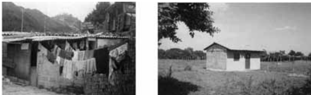
Figure 3. Left: Informal dwelling in Bogotá. The progressive improvement in materials and technologies increase the value of the property (the sign reads: “on sale”). Right: Free standing unit in La Paz, El Salvador, characterized by the box-effect and four-façade uniformity in technology and materials.
