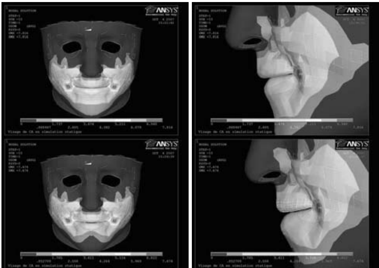
Figure 2 Simulation of smiling lips without (top panels) and with (bottom panels) handling of lips-teeth and upper-lower lips contacts. Displacements are in mm.
