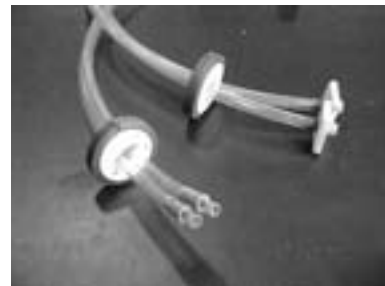
Figure 1: Acoustic wave guides and their suspension arrangement
