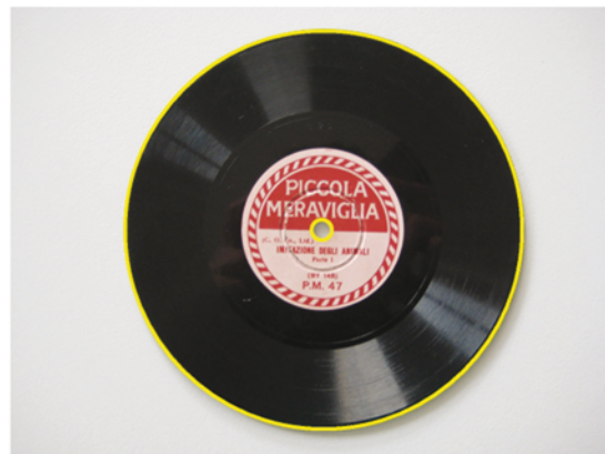
Figure 3. Disc and spindle hole contours automatically detected via the integrodifferential operator.
