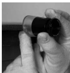
Fig. 11 – Measuring consecutive rings using a manual magnifying glass with a scale inside.
