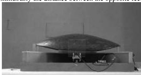
Fig. 20 – The shield 408 mounted on the apparatus: side view, showing the longer (“vertical”) diameter. The shield lays on a plastic soft cushion, the feelers press very gently on its edge. The data logger’s memory, when measuring rate is set at 15 minutes, has a capacity of about 96 days. The battery can last over 1 year.
