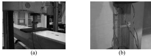
Fig. 1. Test set-up for destructive tests: (a) compression parallel to the grain; and (b) tension parallel to the grain.
