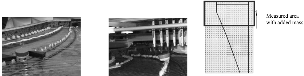
Fig. 7 Artificial added mass on the soundboard
