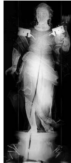
Fig. 8 – Anjo Ceroferário . X-ray examination of whole sculpture, where we can see an internal long longitudinal crack.
