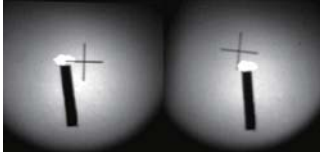
Figure 5: A pair of stereoscopic images of a rectangle slit in a thick paper
