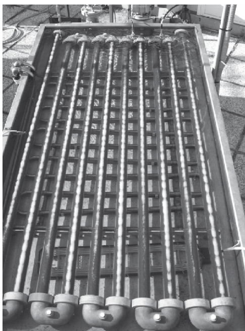
Figure 34. General view of the 50 L horizontal tubular photobioreactor used for outdoor hydrogen experiments with Rhodospseudomonas palustris 42OL.
