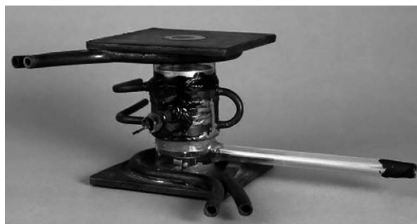
Fig. 6 – First Magnetron prototype developed at Birmingham in 1940.
