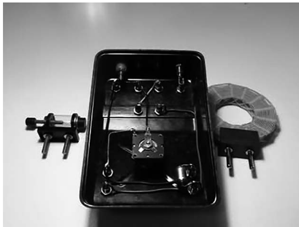
Fig. 3 – Crystal radio receiver. ( top ) Radio receiver schematic diagram. ( bottom ) A radio receiver set on the left the cat's whisker detector is clearly visible.
