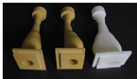
Fig. 3: Three different mechanical vocal tracts obtained using a 3-D printer. All share the same area function but with a different geometrical approximation: (from left to right: case 1: circular and centered shape, case 2: circular ecentered shape and case 3: elliptical centered shape).
