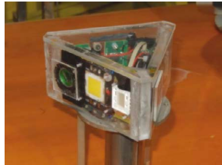
Figure 2 – Optical modem detail: omni-directional light head.
