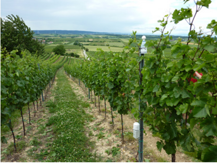
Figure 13.2: Transect measurement station of vineyard climate (air and soil temperature, relative air humidity, potential evaporation) in hilly Austrian terrain (compare derived results of Fig. 12.4 and Fig.8.11 in the other chapters); (source: BOKU-Met).
