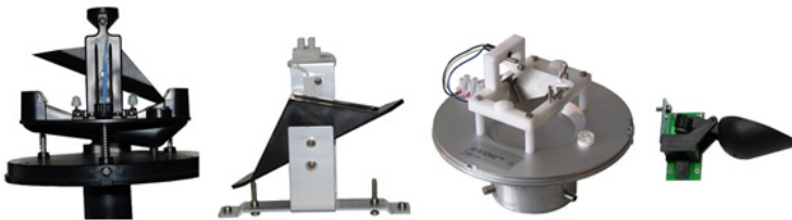
Figure 13.11: Various rain gauge (tipping bucket) mechanics (Source: Pacher).
