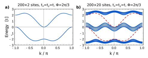
Figure 2.6: Energy bands for (a) a two-leg ladder with  $200 \times 2$  lattice sites (PBC along the long dimension) pierced by a magnetic flux  $\Phi = 2\pi/3$  per plaquette (b) a bigger ladder having  $200 \times 20$  sites. The two-leg ladder bands exactly reproduce the edge states energy of the the bigger ladder (red dashed lines). The two spectra have been calculated diagonalizing the Hamiltonian 2.25 in the "unphysical" gauge with the software *Mathematica*.
