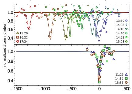
Figure 3.6: Clock laser spectroscopy of a spin polarized  $^{173}$ Yb gas confined in a 3D (s=30) optical lattice. **a:** spectroscopic measurement performed with the clock laser not referenced to the ultrastable 1542 nm frequency reference provided by INRiM show an apparent shift in time of the resonance position due to the aging drift of the ULE cavity which stabilize the laser frequency. **b:** the stabilization of the clock laser on the 1542 nm optical reference
