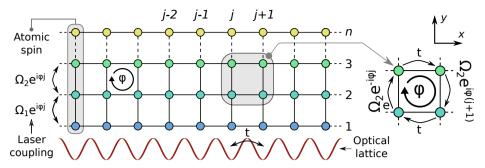
Figure 2.7: Sketch of the synthetic ladder realized combining a one-dimensional optical lattice with an internal atomic degree of freedom, such as, for example, the spin. Laser radiation provides the synthetic coupling in the artificial dimension. Atoms tunnelling along the synthetic lattice pick up a phase that depends on their position in real space, as if they are influenced by a vector potential.
