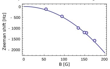
Figure 6.1: Second order Zeeman shift of the clock transition in <sup>174</sup>Yb. The solid line is a fit of the experimental data with a parabolic function.
