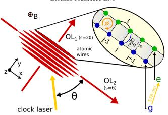
Figure 4.5: Sketch of the experimental setup used for the observation of the chiral currents. An array of fermionic wires is realized confining the atoms by means of two deep lattices  $OL_1$  and  $OL_3$ , (not shown, in the plane orthogonal to the picture). Each wire is a realization of a two-leg hybrid ladder in the synthetic dimension picture. The angle  $\theta$  at which the clock laser intersects the wires defines the synthetic flux  $\Phi$ .
