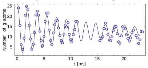
Figure 3.5: Rabi oscillation between the electronic states  $^1S_0$  and  $^3P_0$  relative to a spin polarized  $m_F=-5/2$  atomic sample trapped in a  $s=30\,E_r$  isotropic 3D optical lattice.
