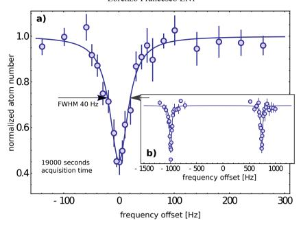
Figure 3.7: **a:** Long-term addressing of the clock transition (5.2 hours). The error bars indicate the standard deviation of the mean over approximately 10 repeated measurements. The lines are fits with Lorentzian functions. The zero values for the horizontal scales are chosen arbitrarily. **b:** Clock transition relative to the  $m_F = \pm 5/2$  spin state. The mean value of center of the two resonances is used to extract the absolute value of the clock transition. frequency (see text).
