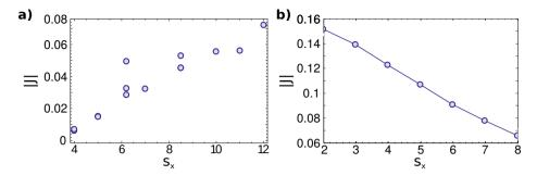
Figure 5.5: Chiral currents dependence on the lattice depth  $s_x$  for the experimental parameters  $\Omega_1^R/t=3.7$ ,  $f_x=2\pi\times55$  Hz. The theoretical prediction based on DMRG simulation performed by the group of R. Fazio in Pisa (**b**) is compared with the experimental data (**a**).
