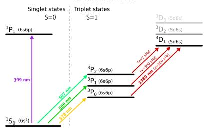
Figure 1.1: Scheme of the lowest energy Yb levels. Also the repumping transitions connecting the  $^3P$  (6s6p) multiplet with the  $^3D_1$  (5d6s) state are shown.
