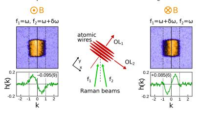
Figure 5.4: Time-of-flight images of the momentum distribution n(k) and asymmetry function h(k) = n(k) - n(-k) of the  $-\frac{1}{2}$  spin state in the two-leg ladder configuration for opposite values of the effective magnetic field. The sign of the magnetic field is changed swapping the frequency of the two Raman beams. Experimental parameters adopted in the experiment:  $\Omega_1^R = 2\pi \times 394$  Hz,  $t = 2\pi \times 87$  Hz and  $\Phi = \pm 0.37\pi$ .
