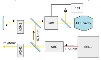
Figure 1.3: Conceptual scheme of the 578 nm laser setup. See the main text for details.
