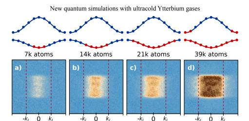
Figure 1.11: **a-d:** Band mapping for several fillings for a 3D lattice with depths  $s_{x,y,z} = \{6,30,30\}$ . On the top of each panel a sketch of the filling of the fundamental and first excited bands is shown. The square shape in the last panel correspond to the FBZ (integrated along the vertical axis).
