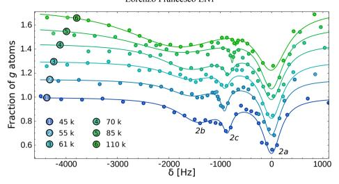
Figure 6.8: Clock spectroscopy as a function of the atom number performed in an anisotropic 3D lattice characterized by the depths  $s_{x,y,z} = \{15, 30, 15\}$ . An additional peak (labelled as 2c) is revealed between the peaks 2b and the blue sideband (2a) as the atom number is reduced (see the main text for details). Frequency offsets are given with respect to the peak 2a.
