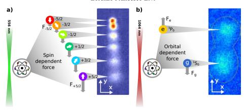
Figure 1.7: **a:** Example of OSG detection on a SU(6)  $^{173}$ Yb spin mixture. Spin dependent force is exerted by a 556 nm beam, 566 MHz red-detuned with respect to the MOT frequency. **b:** Example of simultaneous detection of atoms in the orbital states  $^{1}S_{0}$  and  $^{3}P_{0}$ . Orbital dependent force is exerted by a 1064 nm beam slightly misaligned with respect to the trap.
