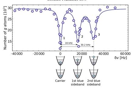
Figure 3.3: Sideband-resolved spectrum of the clock transition of a spin polarized  $^{173}{\rm Yb}$  gas trapped in a 3D lattice with a depth  $s\simeq 22$ . In the spectrum, in addition to the carrier transition, it is possible to observe the first two lattice blue sidebands. The absence of red sidebands implies that all the atoms occupy the fundamental lattice band before the clock excitation. The frequency spacing between the peaks matches the spacing between lattice bands at  $s=22\,E_R$ .
