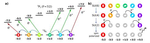
Figure 1.6: **a:** Scheme of the optical pumping processes employed to generate SU(N) spin mixtures.  $\sigma^+/\sigma^-$  processes indicated with a solid arrow are performed before the final evaporation of the gas. Blast pulse indicated with a red arrow are instead performed after the final evaporation. **b:** Sketch of the experimental sequence used to generate SU(4), SU(2) mixtures or spin polarized gases starting from a SU(6) unpolarized spin mixture.
