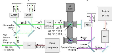
Figure 1.2: 556 nm and 399 nm lasers locking scheme on Yb atomic reference. The labels on the laser beams report the shift in MHz with respect to the light exiting from the doubling cavities (in the 556 nm setup, B and F refer, respectively, to the shifts of the bosonic and fermionic setup. See the main text for details. All the AOMs are in double passage.
