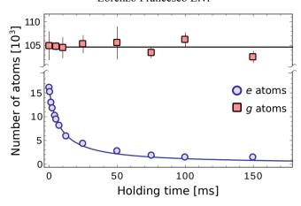
Figure 6.13: Experimental characterization of the loss rates associated to inelastic e-e collisions Number of e atoms (circles) and g atoms (squares) as a function of the holding time in the lattice after a clock excitation pulse in an 1D lattice. The upper line represents the mean value of g atoms, while the lower line is the result of a fit to the e data with the model in equation (6.23), assuming the scaling in equation (6.30).
