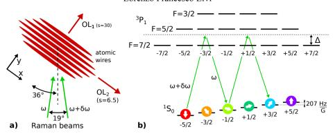
Figure 5.1: **a:** Scheme of the Yb levels involved in the Raman transitions. The value of the Raman detuning is  $\Delta = 1.876$  GHz. **b:** Sketch of the experimental setup showing the relative position of the Raman beams with respect to the optical lattices and the one dimensional fermionic tubes.
