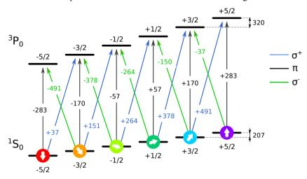
Figure 3.1: Diagram of all the possible transitions connecting the ground state  $|^{1}S_{0}\rangle$  magnetic sublevels with the metastable state  $|^{3}P_{0}\rangle$  sublevels in  $^{173}$ Yb. The first-order Zeeman shifts are calculated with respect to the absolute value of the frequency transition and are reported in Hz/G.
