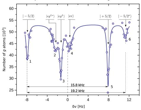
Figure 3.4: Clock transition spectrum of an SU(2)  $^{173}$  Yb sample (spin  $m_F=\pm 5/2$ ) trapped in a s=30 isotropic 3D lattice. For the identification of the peaks see the main text.
