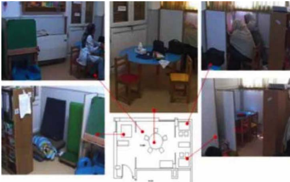
Figura 07. Planimetria della compartimentazione di una classe speciale progettata da Magda Mostafa nella sperimentazione presso l'Advance Society for Developing Skills of Special Needs Children in Cairo (source: Mostafa, M. (2008) An architecture for autism: Concepts of design intervention for the autistic user, in ArchNet-IJAR : International Journal of Architectural Research , vol.2(1), pp. 189–211 - Copyright to Progressive Architects, Magda Mostafa)
