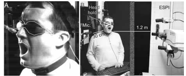
Fig. 2 Measurement settings. A) Detail from measurement camera with highlighted analytical area (mask). B) Position of ESPI and body with head holder and microphone.
