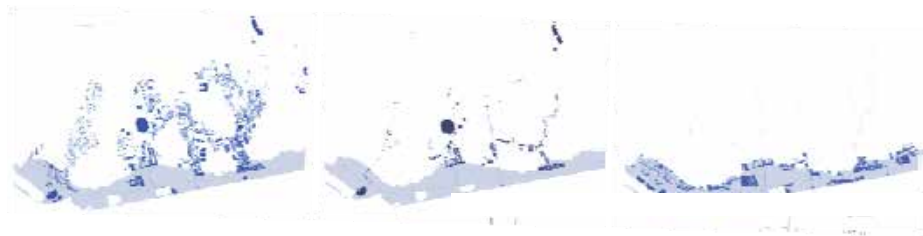
Figure 1 - Map of the elements exposed to risk for the expected sea-level rise (1 buildings at risk of instability: location on slopes starting from water channels up to 100 m away; 2 buildings at risk of submergence: placement within river channels - depressed areas; 3 flood risk buildings: location in the first 5 m of the frente starting from the river).
