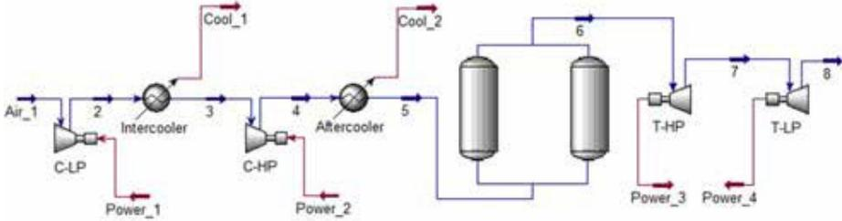
Figure 6 - Plant layout of a CAES system.
