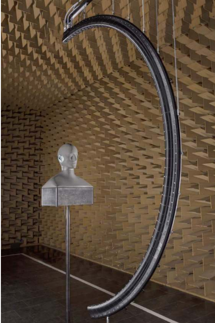
Figure 3.4: Full HRTF measurement setup from behind. Exemplary measurement of an artificial head.
