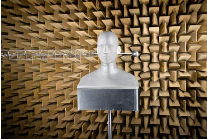
Figure 2.6: HRTF measurement of an artificial head using the measurement arm of the Institute of Technical Acoustics.
