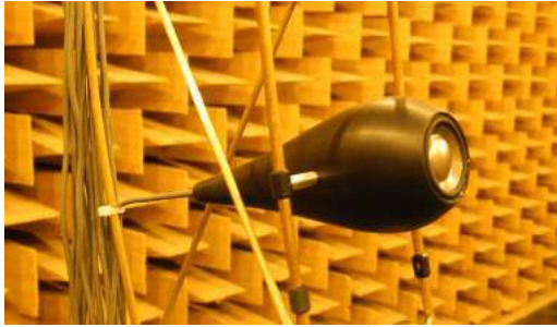
Figure 3.1: Close up view of one loudspeaker in a drop shaped enclosure as employed in the first measurement setup [96].
