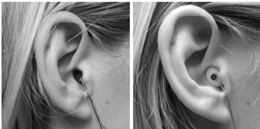
Figure 2.4: Fitting of a miniature microphone with either an open ear canal (left) or closed using an ear plug (right) [21].
