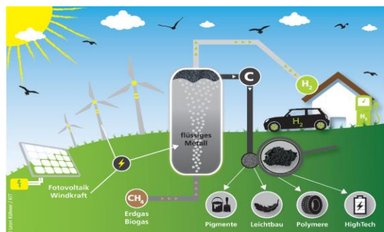
Figure 6: Graphical illustration of methane pyrolysis using bubble column reactor. (Infographic: Leon Kühner, KIT) [4]
