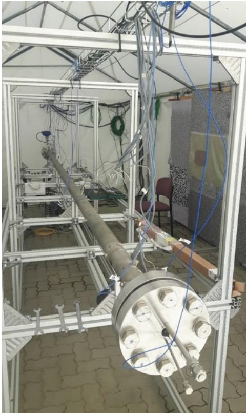
Figure 10: CRYOTUBE experiments mounted on a rack for the ambient warm pre-cursor tests.
