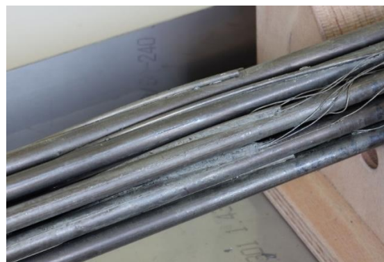
Figure 3: Complete blockage of two sub channels for the experiments in EU-Project MAXSIMA, wires are part of the temperature sensor instrumentation within the blockages and the surrounding rod walls.
