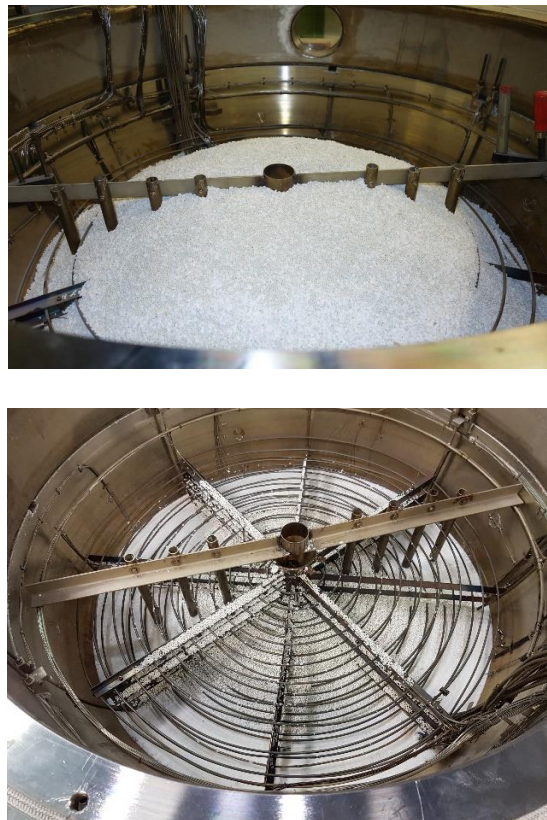
Figure 3. Appearance of initial debris bed (top) and the debris bed after the test (bottom) in LIVE-J1 test.
