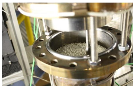
Figure 5: Packed-bed thermocline storage in the pre-experiment VESPA at KALLA (Photo: F. Müller-Trefzer)
