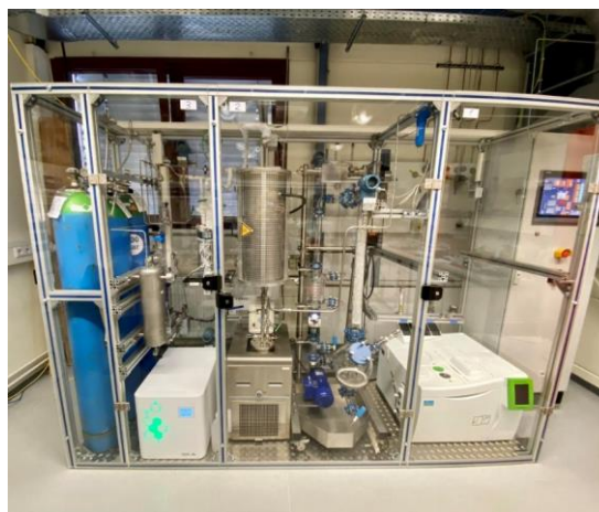
Figure 7: MEDENA set-up for the dehydrogenation of methanol to anhydrous formaldehyde at KALLA (Photo: M. Kamienowska)
