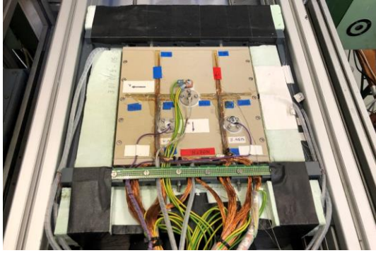
Figure 20 Photo of the instrumented test section partially thermally insulated before insertion in the magnet gap of the MEKKA laboratory.
