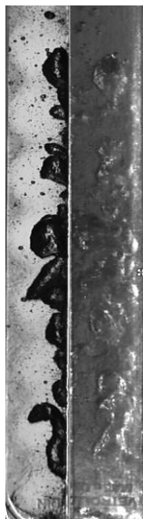
Figure 3 Instant image of the heated section shortly before the boiling crisis (l) and immediately after the power discharge (r).
