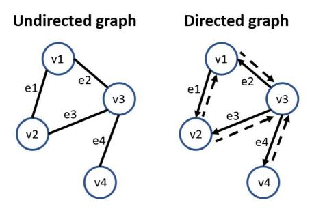
**Figure 12.1:** a) Undirected graph, where vertices or nodes are connected with bidirectional edges. b) Directed graph, where vertices or nodes are connected with directed edges represented by arrows. Arrow's tail points the source and the arrow's head points to the sink.
