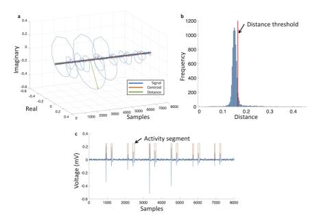
**Figure 11.2:** Electrogram activity detection in the Hilbert space. a) Electrogram signal (c) in the Hilbert Space with centroid (orange trace), green arrow depicts the distance measured from the centroid to the signal. b) Frequency distribution of centroid to signal distance, red line represents mean value plus one standard deviation. c) Bipolar electrogram (blue trace) and activity segments (orange trace). Adapted from [118].
