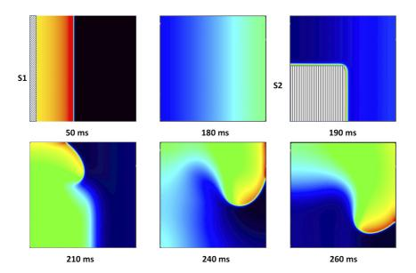
**Figure 8.1:** Snapshots in time explaining the cross-schock (S1-S2) protocol. The first panel (left upper corner) shows the S1 pulse and the depolarization wave. At 180 ms, the tissue cells are finishing their repolarization phase, and then at 190 ms, a second stimulus (S2) was introduced in the lower left quarter of the tissue to induce a reentry. From the time 210 ms, it is possible to observe the reentry activity's progression and maintenance in the cardiac tissue.
