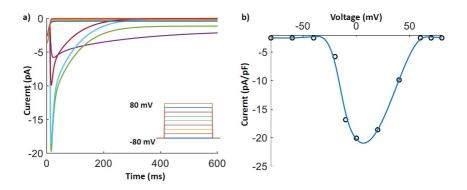
**Figure 7.1:** Fitted myofibroblast  $I_{CaL}$  according to experimental data. a) Voltage clamp experiments of the  $I_{CaL}$  where the behavior of the current is shown at different voltages. b) White dots represents the maximum current value of  $I_{CaL}$  with respect to the experimental data[79] (blue curve).
