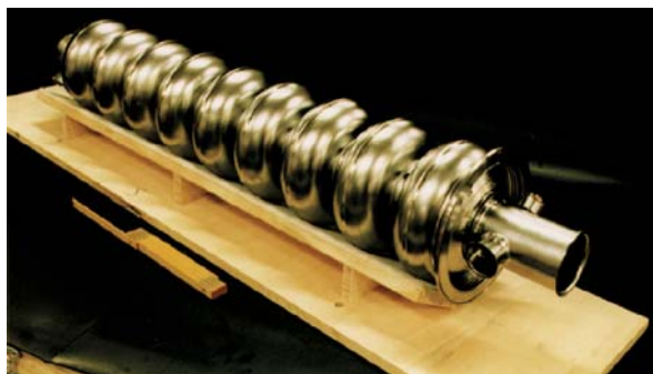
Fig. 3.24 Superconductive accelerating cavity in niobium for the acceleration of electrons. Niobium is superconductive at the temperature of liquid helium. This resonator was designed for the TESLA test facility. Photograph from [13], with permission
