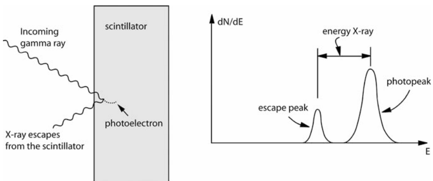
Fig. 6.18 Escape peak: a gamma ray interacts in the scintillator and ejects a K-shell electron from one of the atoms. If the resulting K-shell X-ray escapes from the scintillator, this gives rise to a peak corresponding to the total energy minus the energy of the X-ray. In NaI, the energy of these X-rays is 49.1 keV
