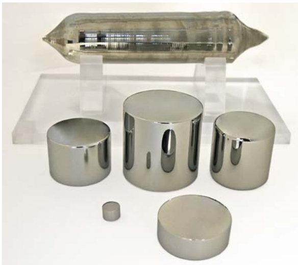
Fig. 5.14 Germanium ingot and Ge detector elements. Figure by courtesy of CANBERRA – an AREVA company
