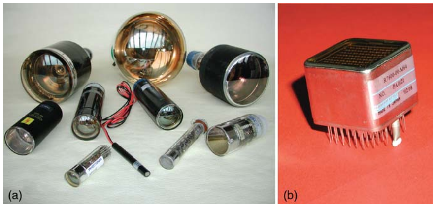
Fig. 6.10 (a) Collection of single channel photomultiplier tubes of various diameter. The largest tube in this image has a diameter of 20 cm. (b) Multi-anode PMT from Hamamatsu with 8 \times 8 independent small PMTs in one single vacuum enclosure. The tube measures 25 \times 25 \text{ mm}^2
