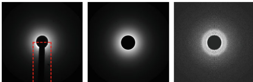
Fig. 8.5 Diffraction images from \text{CBr}_4 doped helium droplets. Left: Raw image from \text{CBr}_4 doped helium droplets, Middle: Wiener filtered regenerated image from left one by refilling the portion inside the dashed box with data from the opposite side of the box and averaging over all four quadrants, Right: image after droplet background removal. Reprinted from “Electron diffraction of \text{CBr}_4 in superfluid helium droplets: A step towards single molecule diffraction”, J. Chem. Phys. 145, 034,307 (2016), with the permission of AIP Publishing
