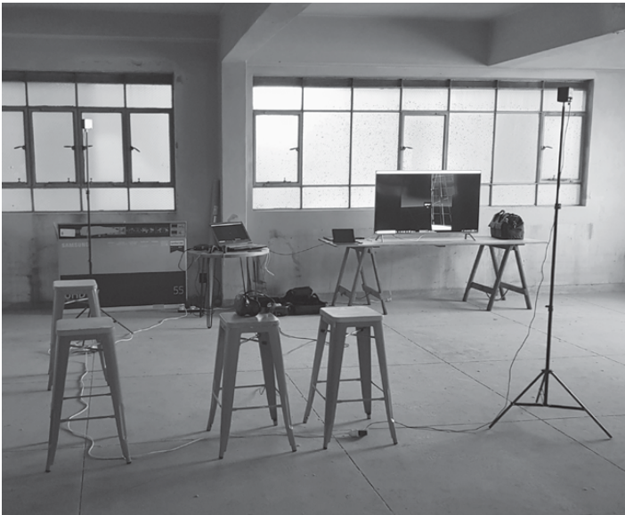
Figure 1.2: VR demonstration set up for public display. Note the tracking beacons mounted on tripods at the edges of the game area creating a trip hazard of trailing wires, here fenced off with a collection of stools
