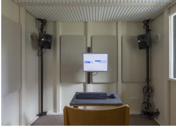
Figure 4.1: ITA sound-attenuated hearing booth
