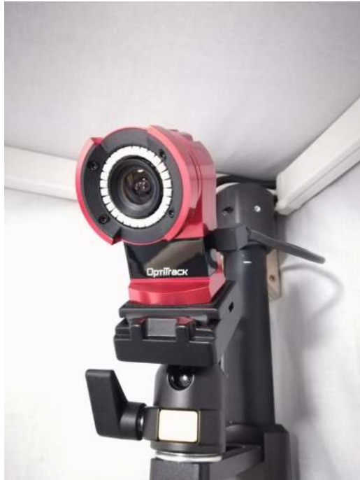
Figure 4.3: Camera OptiTrack Flex 13, with 1.3 million pixels of resolution and 120 FPS sample rate
