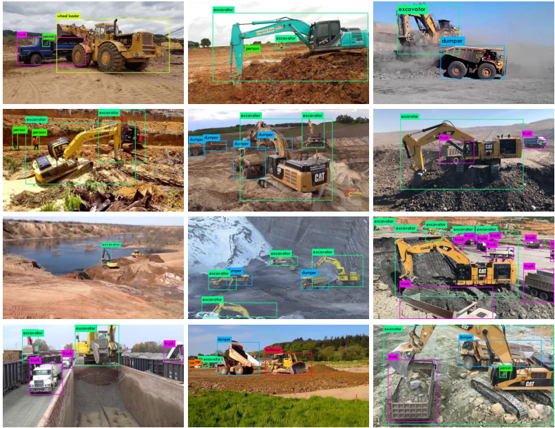
Figure 6.8: Prediction samples with optimized dataset and algorithm YOLOv3.
