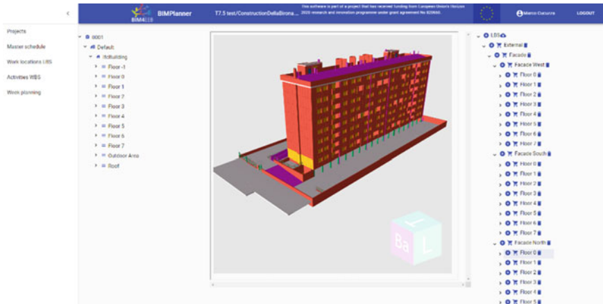
Fig. 6.14 BIMPlanner work location LBS page: upload of the fully panelised IFC model
