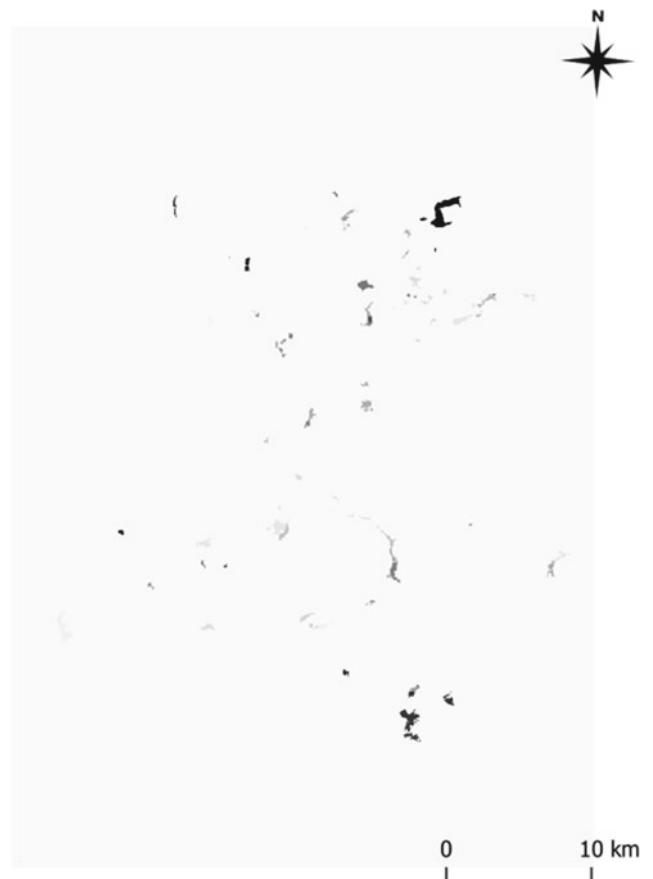
Fig. 16 Result from Exercise 4. Raster displaying the areas that are different in the two maps compared, that is, the areas of change in the time series
